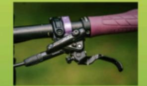
When the levers are squeezed, the brake pads press against the wheels and due to friction it slows the motion of the bike. Chain rings Rear Derailleur Chain Que Chain Chainset
